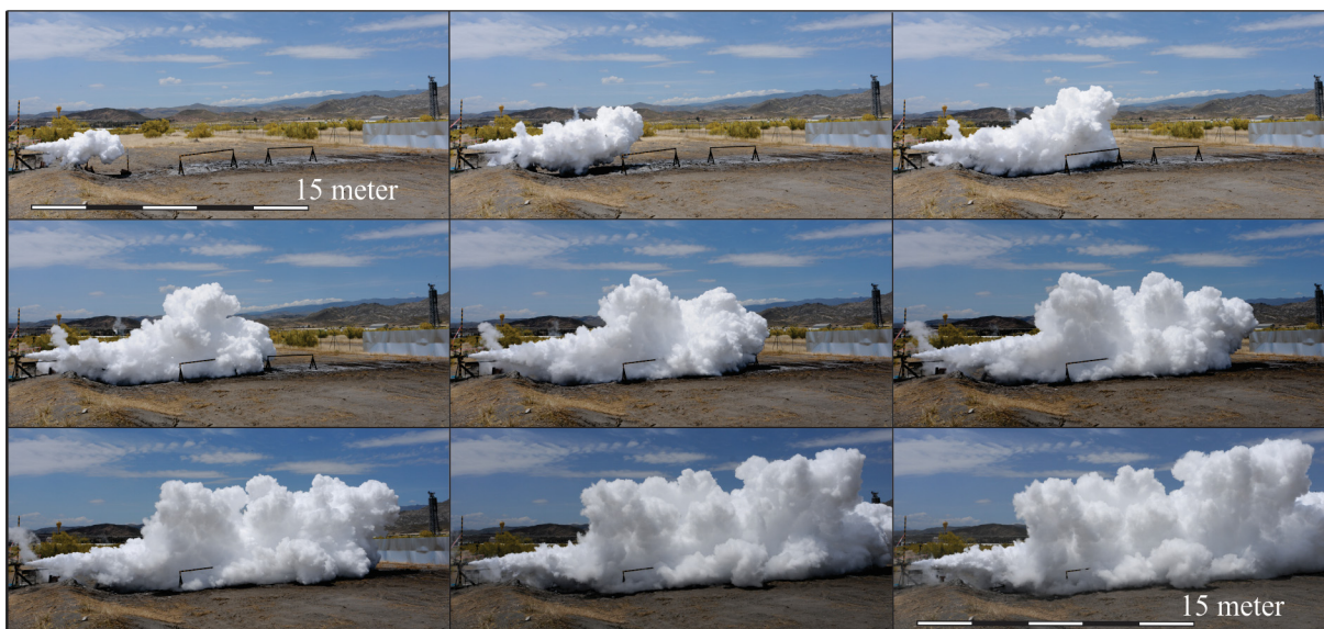
FIGURE 10. Photo series taken during the first 3 seconds (3 pictures / second) of the 2" HELISOL ® 5A release test at 420 °C
