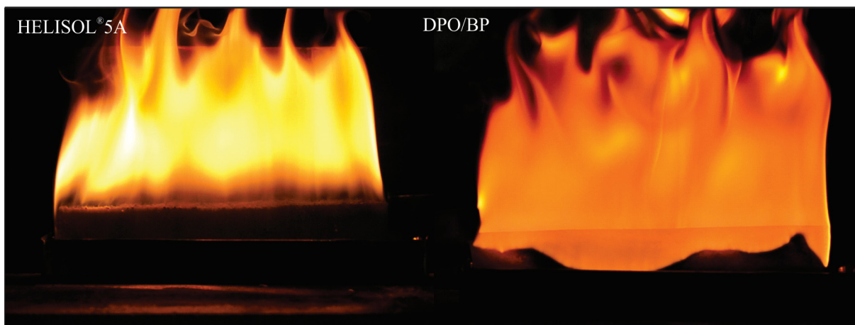
FIGURE 3. “Wick flame test” according to DIN EN ISO 14935, left side HELISOL® 5A, right side DPO/BP. Both wicks caught fire entirely and remained burning for more than 60 seconds.
