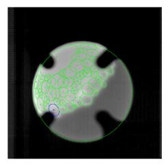
FIG. 9. Image taken from the high-speed camera video during solidification of a  $Al_{75}Ni_{25}$  sample upon an undercooling of 291 K prior to solidification using the EML on board the ISS. The green circles adumbrate the crystals which are formed by copious nucleation in front of the propagating solid-liquid interface. The first nucleation event was on the upper left side (large circle). Evaluation of experiments performed on board the International Space Station in June 2017.
