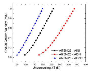
FIG. 4. Dendrite growth velocities as a function of undercooling of the various phases involved in the solidification of undercooled  $Al_{75}Ni_{25}$  alloy, AlNi (black),  $Al_3Ni_2$  (blue), and  $Al_3Ni$  (red).
