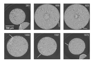
FIG. 10. Selected synchrotron x-ray microtomography slices of a  $310-\mu$ m Al<sub>80</sub>Ni<sub>20</sub> droplet atomized in helium. The arrows denote nucleation points at the surface of the droplets with primary dendrite arms growing towards the center of the droplet.
