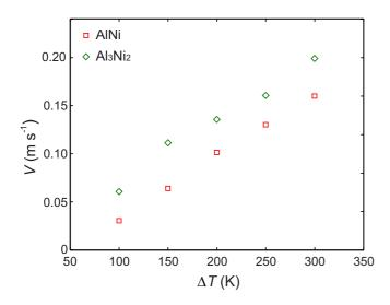
FIG. 5. Calculated growth velocity as a function of undercooling estimated from the coupled thermosolutal phase-field model. Calculation shown for primary growth of both AlNi and of  $Al_3Ni_2$  in an undercooled melt of the  $Al_{70}Ni_{30}$  alloy.
