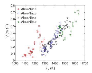
FIG. 7. Growth velocity for Al-*x* at. % Ni (x = 25, 30, 31.5, and 35) as a function of nucleation temperature,  $T_N$ . Open symbols = inverse velocity trend (*V* decreasing with  $\Delta T$ ); filled symbols = normal velocity trend (*V* increasing with  $\Delta T$ ). Most data follow a single trend with  $T_N$ .
