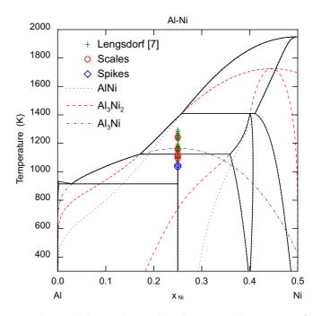
FIG. 1. Al-Ni phase diagram including metastable extensions of the liquidus and solidus lines for AlNi (dot),  $Al_3Ni_2$  (dash), and AlNi<sub>3</sub> (dot-dash) phases. Also shown are the temperatures at which velocity measurements have been made for  $Al_{75}Ni_{25}$  on Earth by Lengsdorf *et al.* [7] and in microgravity.
