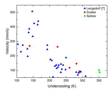
FIG. 2. Dendrite growth velocity as a function of undercooling measured on Earth (triangles) and in microgravity (circles) for alloy Al<sub>75</sub>Ni<sub>25</sub>. Data of the terrestrial experiments are taken from Ref. [7]. The color of the circles denotes the growth morphology observed by the high-speed camera, scales (red) and spikes (green).
