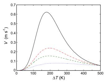
FIG. 6. Exemplary LKT type calculations using undercooling dependent |m| and  $k_E$ . (|m| increasing with  $\Delta T$  and  $k_E$  decreasing with  $\Delta T$ ): Dots: both |m| and  $k_E$  linear; dash: |m| convex down and  $k_E$  linear; dot-dash: |m| linear and  $k_E$  convex up; solid: |m| convex down and  $k_E$  convex up.
