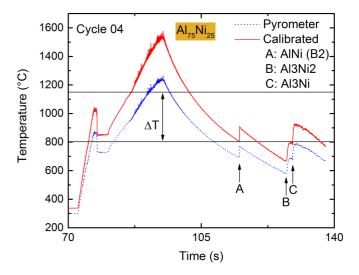
FIG. 3. Temperature-time profile measured during solidification of Al<sub>75</sub>Ni<sub>25</sub> in Space upon an undercooling of  $\Delta T \approx 350$  K. The red curve gives the data of the pyrometer calibrated by the correct emissivity. Three phase formation temperatures are observed labeled A–C.
