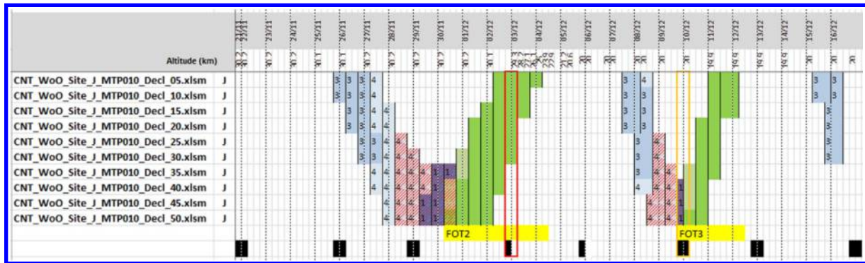
Figure 8. CONSERT WoO summary spreadsheet sample %. Each row corresponds to a specific configuration for Philae, the comet and Rosetta. The columns are the time calendar for one month of operations. Green boxes shows the time span where CONSERT operations are possible with a good science return. Other colors highlight different constraints inadequacy, showing the complexity value of the Philae operation. Black boxes, red and yellow outlines show periods during which operations are not possible because of Rosetta maneuvers. The yellow boxes then show, for a sweep of acquisition conditions, the window of opportunity for CONSERT observation, which will be refined progressively until the actual operations, finally corresponding to one or two specific green boxes.
