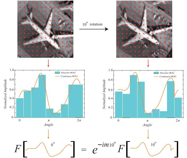
Fig. 3. Illustration of the discrete and continuous HOG distribution function of a cell (13 × 13 pixels). (Left) Reference HOG. (Right) 10° rotated HOG. A property-rotated gap between the two discrete HOGs can be filled by shifting their corresponding continuous HOGs with 10°.
