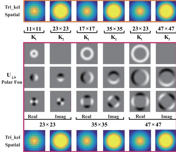
Fig. 5. Triangular convolution kernel of two domains. Spatial [ $K_1$ : the convolution kernel for the spatial aggregation.  $K_2$ : the convolution kernel for the local normalization (based on gradient energy)];  $U_{j,k}$ : the basic function from triangular radial profile and a Fourier basis.
