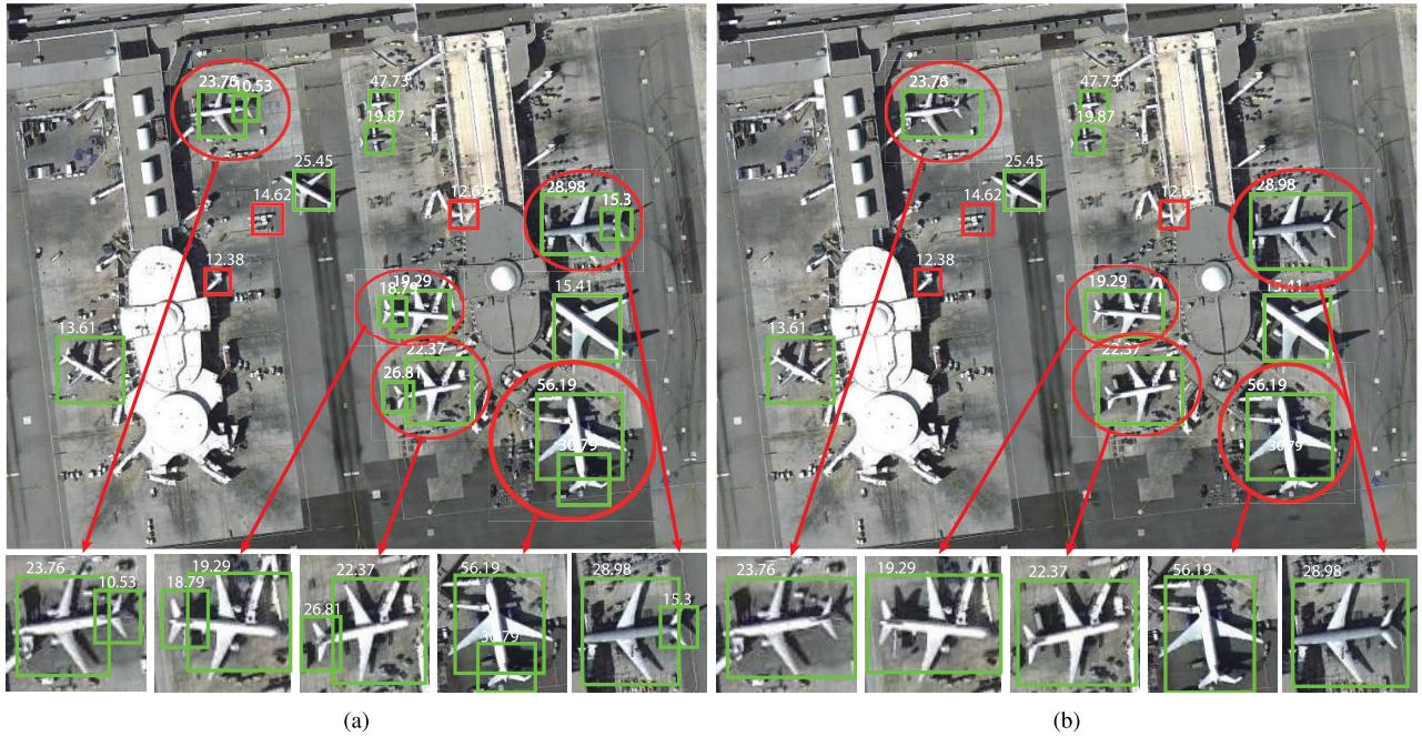
Fig. 9. Overlap removal using original NMS and two-step NMS. (a) Original NMS. (b) Two-step NMS.
