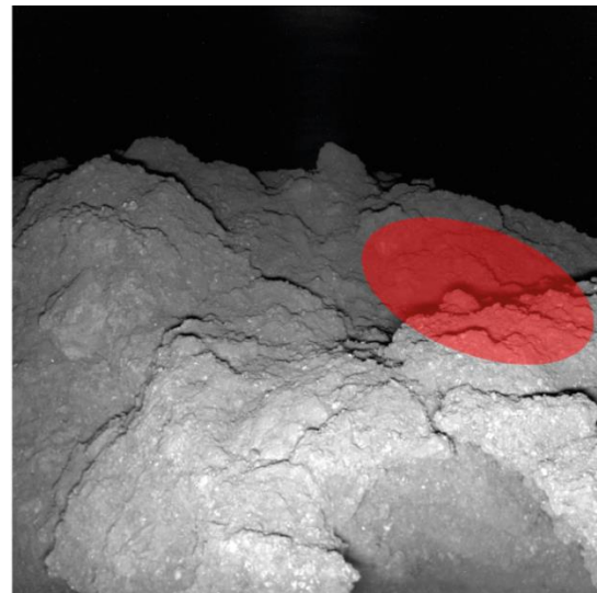
Figure 1 Projection of the radiometer field of view (red ellipse) onto the scene imaged by MASCOT's optical camera. Nighttime image illuminated by the camera's red LED. MARA observes an angular to subangular rock formation. Because of perspective viewing, pixel resolutions vary across the image between approximately 0.2 mm at the bottom and 3 mm near the horizon.
