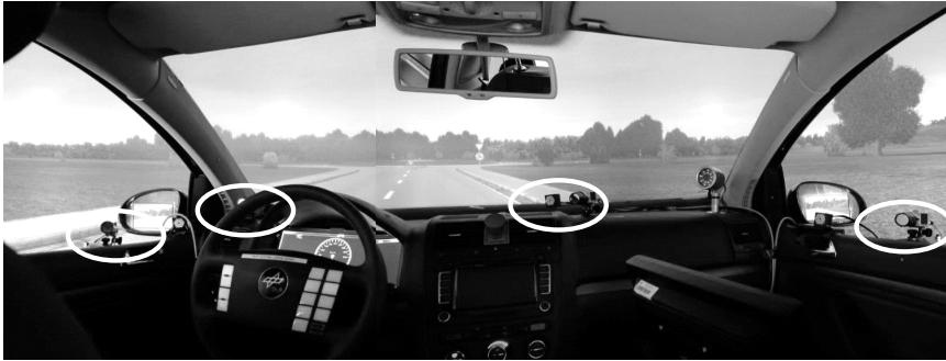
Figure 3-15: Four cameras of the eye tracking system.
