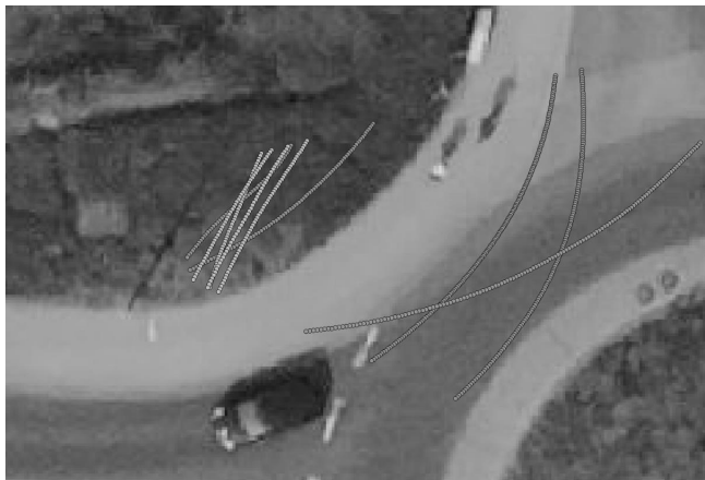
Figure 3-6: Drives with measurement errors detected by checking the first/last yaw values.
