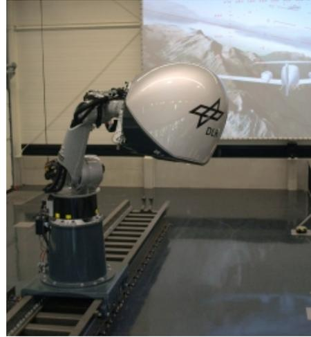
**Fig. 12** Robotic Motion Simulator at the DLR Institute of System Dynamics and Control [2].
