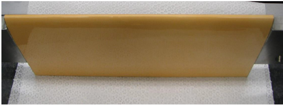
Figure 4: 2D wind tunnel model with TSP coated perforated foil applied to the surface.
