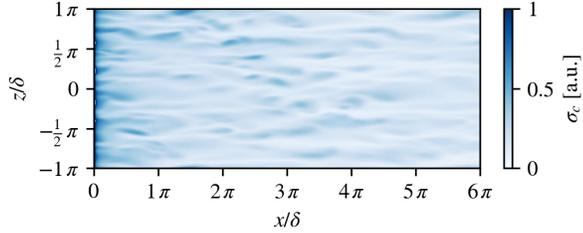
Figure 1: Instantaneous distribution of the vapor source term at the cooled wall. The footprint of the coherent sweeps responsible for wall-normal transport is visible in the pattern of condensation.
