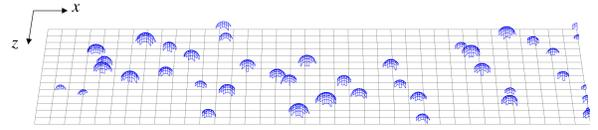
Figure 2: Hemispherical droplets at locations representing regions of high condensate accumulation along the cooled channel wall. Droplet radii are not to scale.
