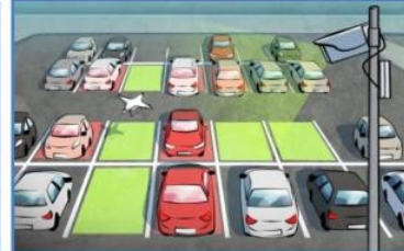
Step 3: Fixed cameras updating parking spot occupancy status
