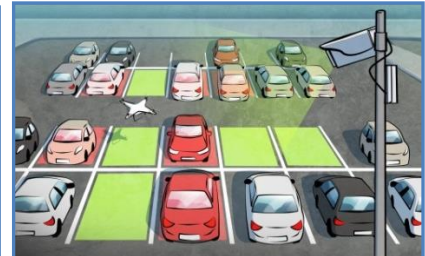
Step 3: Fixed cameras updating parking spot occupancy status
