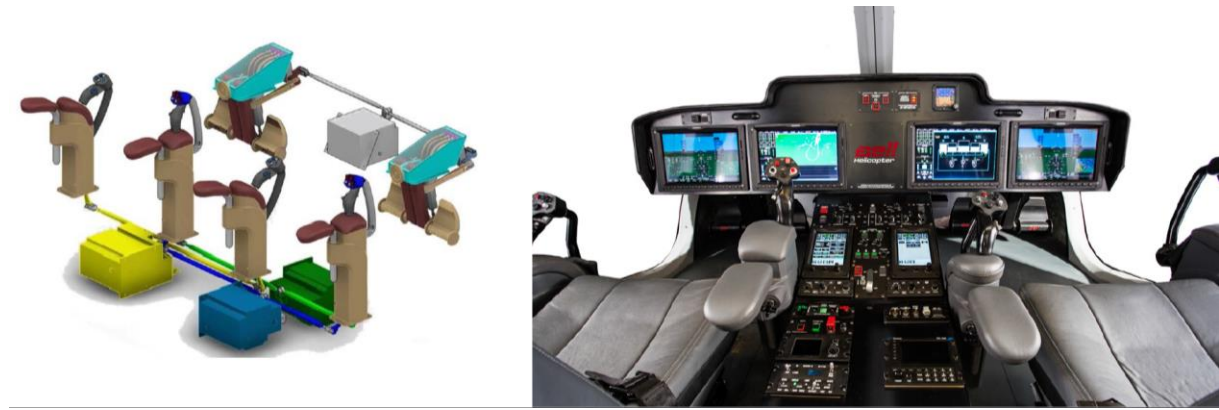
Figure 2.8: Bell 525 mechanically linked flight controls (left) and flight deck (right) [50]
