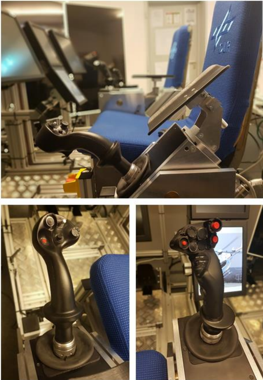
Figure 4.15: Collective grip (bottom left), cyclic grip (bottom right), and 45° collective arrangement (top)
