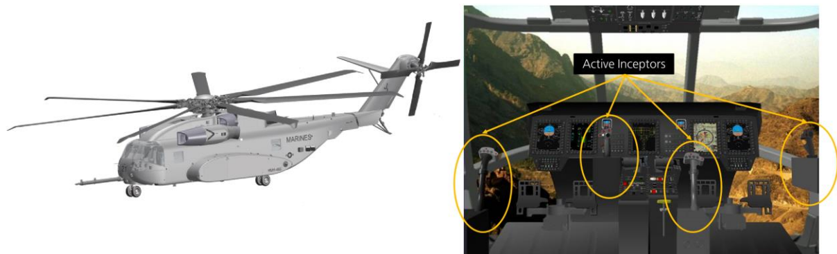
Figure 2.7: CH-53K King Stallion external view (left) and active sidesticks (right) [42]
