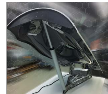
Fig. 4: Eurofighter airbrake demonstrator B-model
