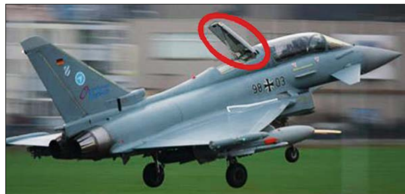
Fig. 1: Eurofighter airbrake, a demonstrator structure for “Structural Bonding Technology” (Source: Airbus)
