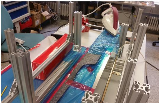
(a) Heating a C-Fin with iron and infrared emitters
