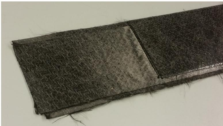
Figure 6.12.: Displacement between plies in the Fin C
