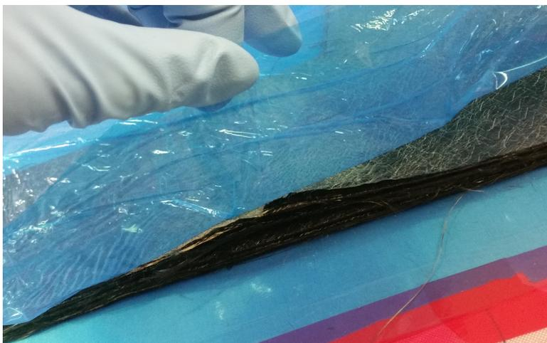
Figure 5.7.: Plies fall out due to an insufficient adhesion
