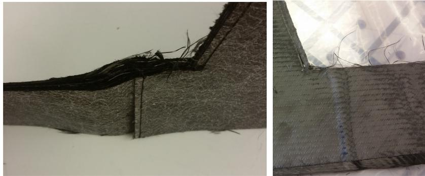
Figure 5.4.: Gap and wrinkle found in the preform
