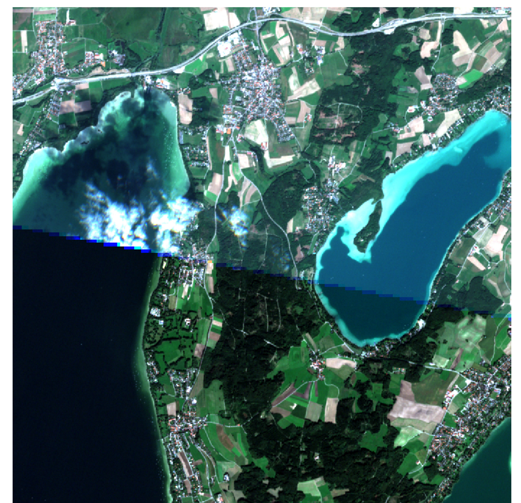
Figure 3. Overlapping satellite images with the reference scene on the bottom half and the corresponding slave scene in the top half.
