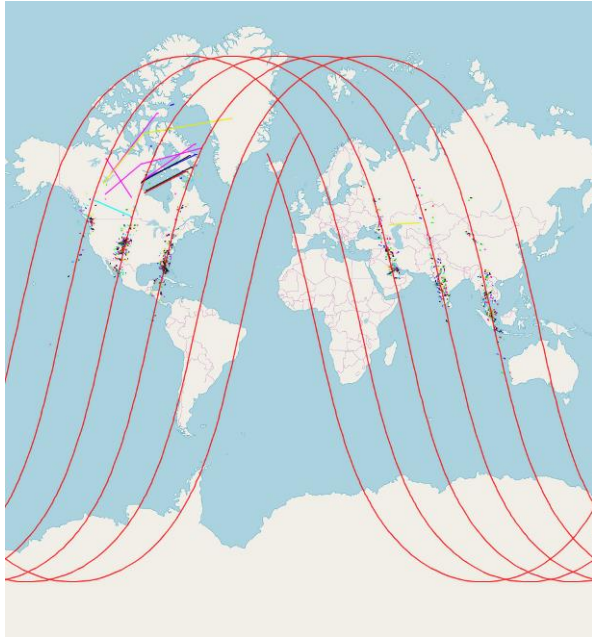
Fig. 3. Example Detection pattern of DLR's in orbit demonstrator with in one track (no accumulation over concurrent tracks) [X1].
