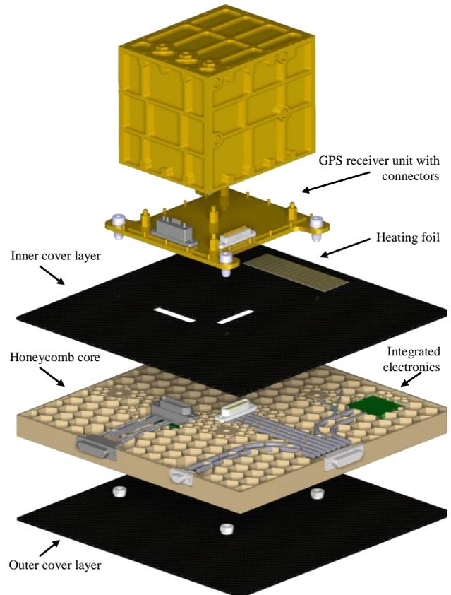
Figure 6. Exploded view of the technology-demonstrator with the GPS receiver unit
