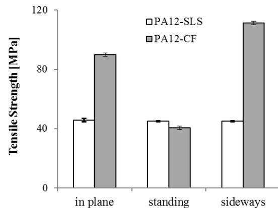
Figure 2. Tensile strength of SLS processed PA 12 (PA12-SLS) and short carbon fiber reinforced FFF processed PA 12 (PA12-CF)
