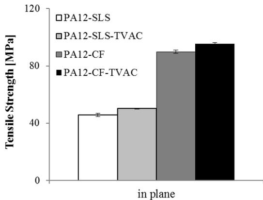
Figure 4. Tensile strength of PA 12 and short carbon fiber reinforced PA 12 before and after (-TVAC) thermal vacuum cycling
