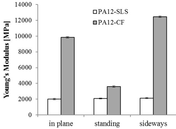
Figure 3. Young's modulus of SLS processed PA 12 (PA12-SLS) and short carbon fiber reinforced FFF processed PA 12 (PA12-CF)
