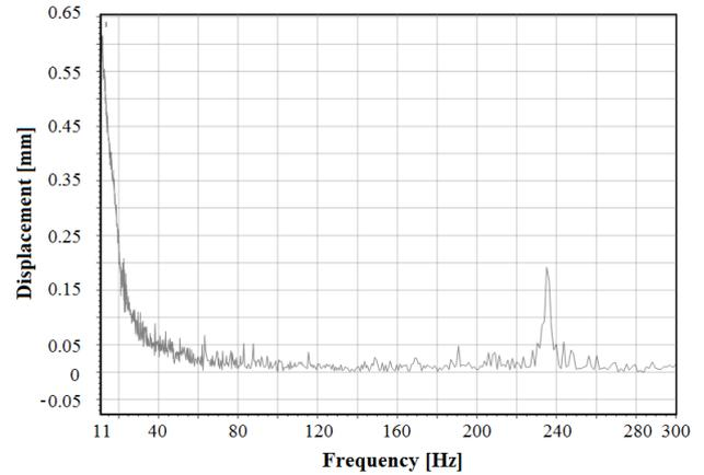
Figure 10. Modal analysis of the test component at 0,3g
