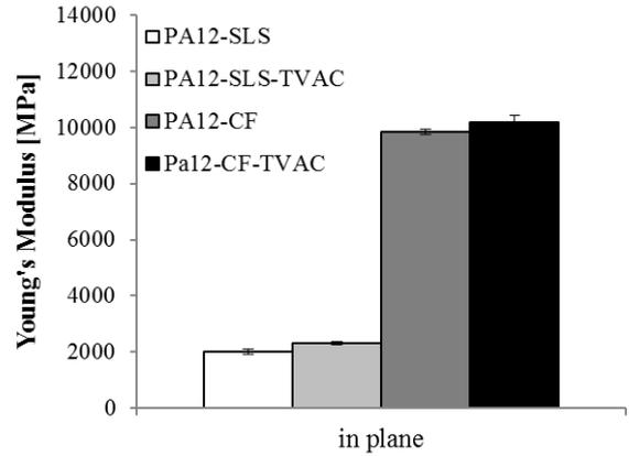
Figure 5. Young's Modulus of PA 12 and short carbon fiber reinforced PA 12 before and after (-TVAC) thermal vacuum cycling
