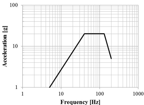
Figure 9. Sine vibration load (HLSS)
