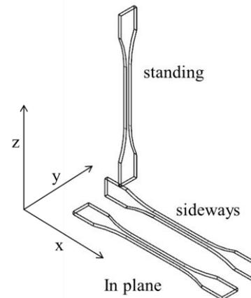
Figure 1. Tensile specimen orientation
