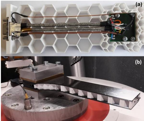
Figure 7. Test component for vibration testing; (a) the printed honeycomb core with integrated electronics; (b) the complete test component mounted on the shaker
