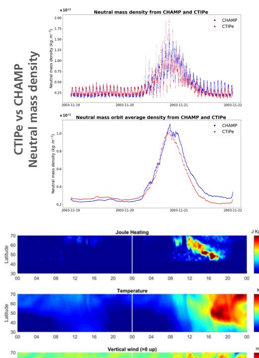
A significant increase of the **neutral mass density** ( $\rho$ ) can be identified in the comparison between values derived from CHAMP [5] (blue) and CTIPe results (red). It was generated by the storm disturbances reaching a maximum one order of magnitude bigger than quiet values.
