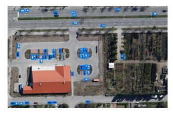
Fig. 3: Vehicle detection result using ShuffleDet on the 3K-DLR-Munich dataset.
