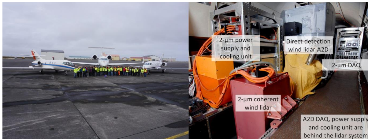
Figure 1. The left picture shows the three aircraft operated during the NAWDEX campaign from the airport in Keflavik, Iceland, namely DLR's Falcon (left), the HALO aircraft (middle) and the French SAFIRE Falcon (right). The right picture illustrates the Aeolus Cal/Val payload integrated in DLR's Falcon aircraft with the 2- \mu\text{m} and A2D DWL including data acquisition unit (DAQ).
