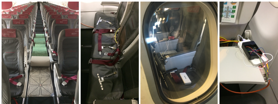
Figure 9. Sensor environment in a field trial environment: sensor floor, seat sensors, central processing unit, seat processing unit (from left to right).
