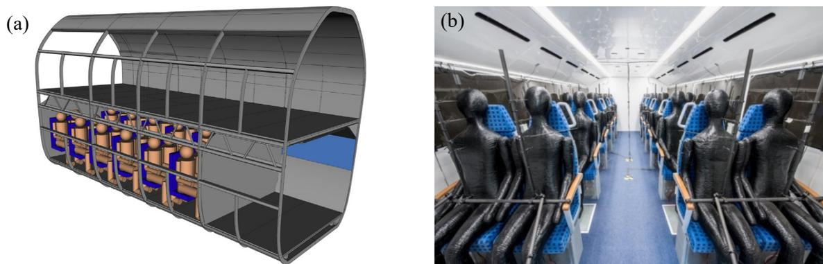
**Figure 1.** (a) CAD sketch of the generic train laboratory. (b) Image of TMs seated in the laboratory. Images © DLR.
