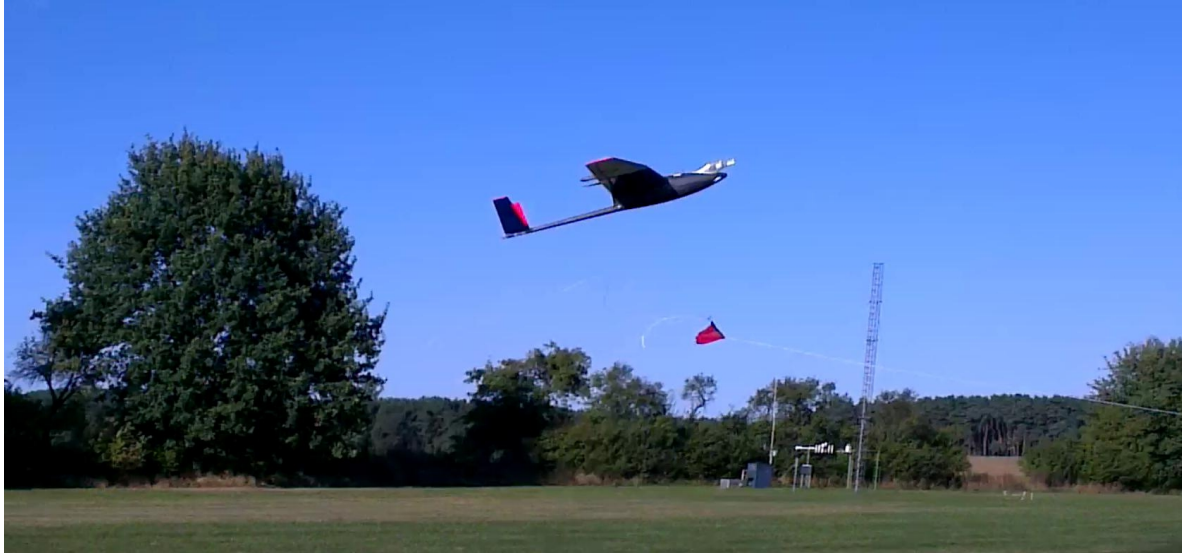
Figure 1. Research unmanned aerial vehicle (UAV) Multi-purpose Airborne Sensor Carrier (MASC) during take-off with a bungee.
