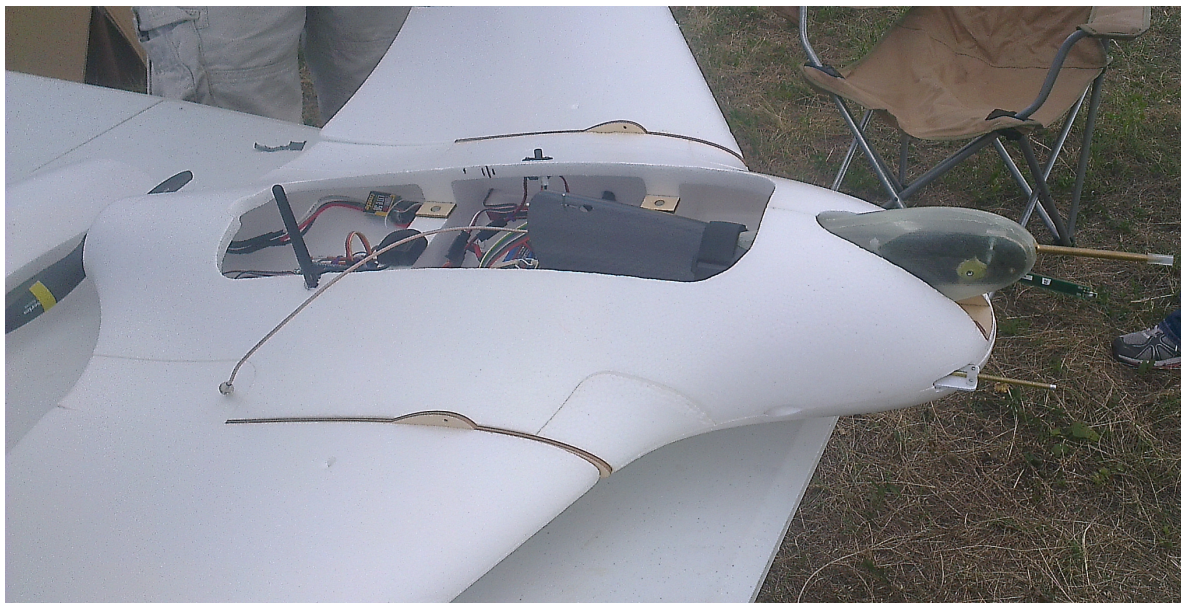
Figure 3. Research UAV Skywalker X8 with the MASC measurement system.
