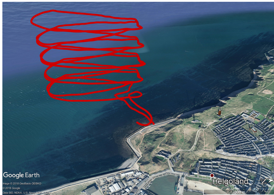
Figure 9. Flight path in red on Helgoland (HEL) on 10 October 2014. The figure shows the flight path on the west coast of Helgoland. The undisturbed marine boundary layer with strong winds from the southeast was measured.
