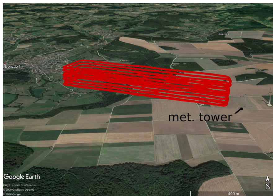
Figure 7. Flight path (so-called racetracks) in red in Schnittlingen (SNT) on 7 May 2015, with the meteorological tower east of the flight path. During the measurement, moderate westerly winds prevailed. The crest forms partial up-drafts and strongly sheared flow.
