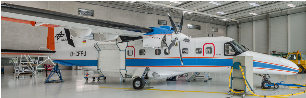
Figure 1.2: DLR's Do228-212 research aircraft with F-SAR system.
