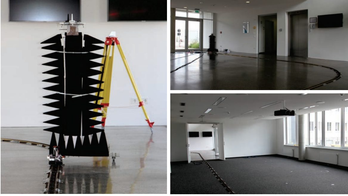
Figure 6.4. Measurement scenario: the left figure shows in front the receiving antenna mounted on the top of the experimental train and in the background the transmit antenna mounted on a tripod. The left figure shows the lobby on top and below the meeting room with the pre-measured tracks.
