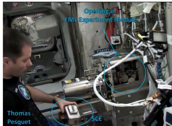
Fig. 4. Thomas Pesquet during SCE installation on-orbit
