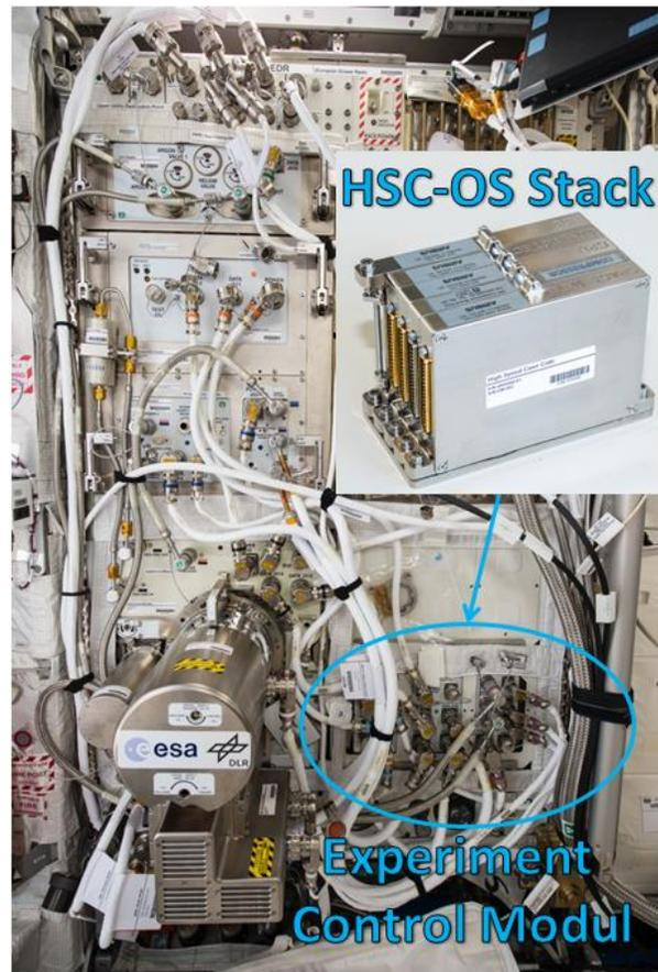
Fig. 5. HSC-OS Stack for integration into EML Experiment Control Modul
