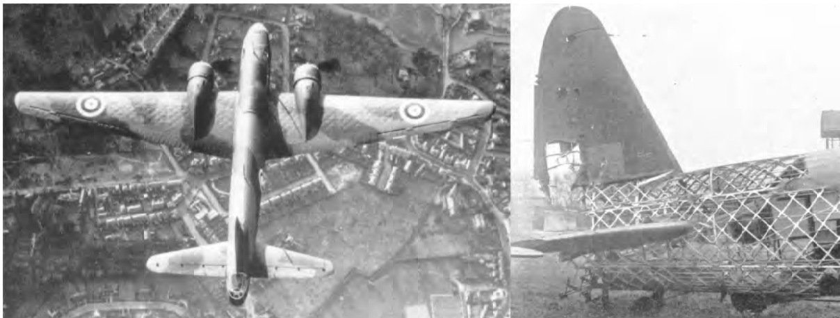
Figure 4: left: Wellington bomber in flight [52] right: Wellington visible structure due to massive damage [52]
