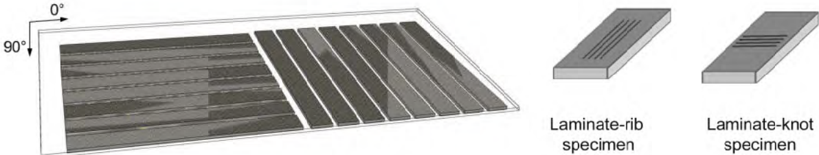
Figure 25: Manufactured thin plate for "laminated" rib and knot specimen [56]
