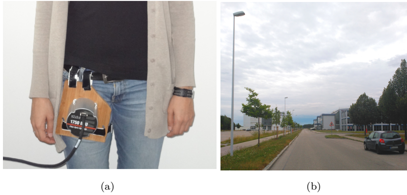
Figure 3.8: (a) The inertial data for the experiments analyzed in this section has been recorded with the IMU DSP-1750 attached to a wooden surface which is fastened to the leg, as if the sensor were introduced in the pocket. (b) Scenario of the experiments detailed in this section.
