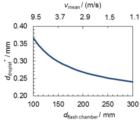
Fig. 6: Diameter of a droplet size that is just being separated from the steam flow by gravity as a function of tube diameter and the steam's mean empty tube velocity.
