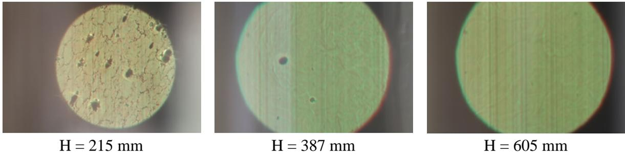
Fig 13: Optical measurements of droplets depending on the column height over inlet position for the same measurement parameters chosen.
