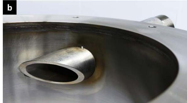
Fig. 4b: Twisted and tangential mounting of the inlet tube.
