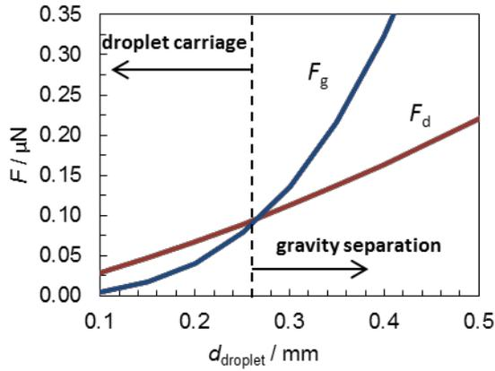
Fig. 5: Forces occurring at the droplet as a function of droplet size in an evaporation tube with a diameter of 200 mm (feed flow 1000 l/h, feed temperature 90 °C, vapor content 4.48 %).
