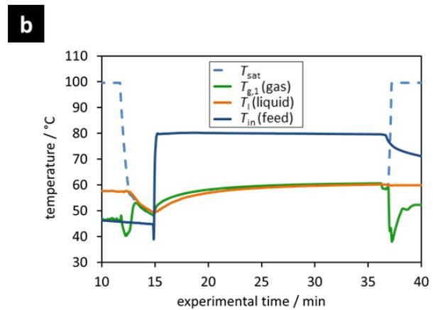
Fig.8a: Evaporation experiment with  $\dot{V}_{\text{feed}} = 1000 \frac{\text{l}}{\text{h}}$ ,  $T_{\text{feed}} = 70 \text{ }^\circ\text{C}$ ,  $p_{\text{flash}} = 240 \text{ hPa}$ , and a flash column diameter of 200 mm. Fig.8b: Corresponding temperature curves.
