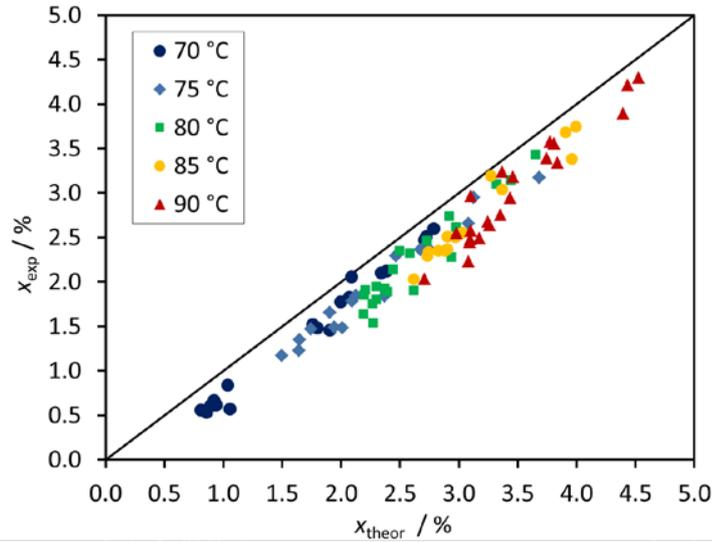
405 Fig. 10: Experimental vapor content versus theoretical vapor yield according to isenthalpic flash evaporation process for varying feed temperatures and volume flows, column diameters of 200 mm and 100 mm, and salt concentrations between regular tap water and 120 g NaCl/l.
