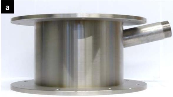
Fig. 4a: Adjustment of the inlet tube to the separation chamber (200 mm diameter).
