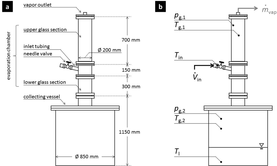
Fig. 3a: Design drawing of the flash chamber. Fig. 3b: Position of measurement points.
