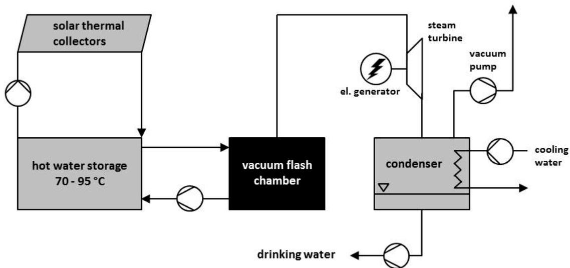
95 Fig. 1: Schematic flow diagram of a multi-effect solar desalination plant as proposed in [15].
