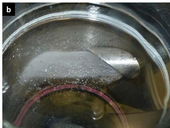
Fig. 12a: Two-phase flow at a feed temperature of 70 °C and a flow rate of 1011 l/h or 0.267 kg/s (200 mm chamber diameter; exposure time: 1/60 s).
