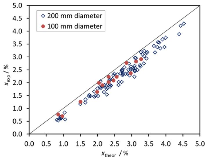
410 Fig. 11: Comparison between different tube diameters according to the experimental vapor content for varying feed temperatures and volume flows, and salt concentrations between regular tap water and 120 g NaCl/l.
