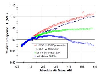
Figure 4: Air mass based correction function by King and Myers [reproduced from (Jessen et al., 2017), p. 9]
