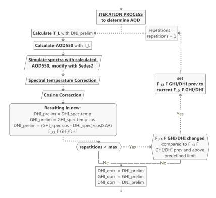
Figure 9: Iteration process of the correction method for the most accurate estimation of the AOD with the available DNI measurement of the RSI.
