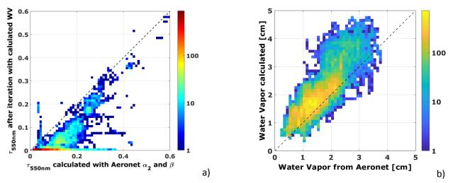
Figure 18: Evaluation of the AOD calculation by (Ineichen, 2008) and calculated precipitable water vapor by (Gueymard, 1993; Gueymard, 1995) for the PSA, Spain. a) Calculated  $\tau_{550nm}$  after the iteration process in comparison with  $\tau_{550nm}$  calculated from Aeronet
