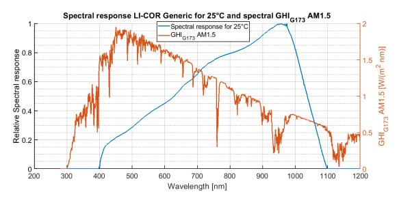
Figure 3: Spectral response of the LI- 200 sensor from (Licor, 2004) under laboratory conditions (assumed to be 25°C) and the GHI spectrum under G173, air mass 1.5 atmospheric conditions (ASTM, 2012).
