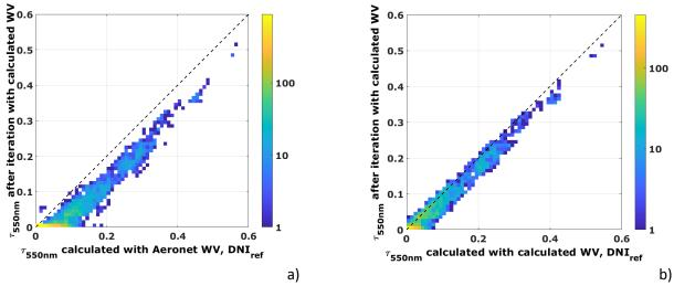
Figure 19: Evaluation of  $\tau_{550nm}$  for sunny time stamps over the course of one year at the PSA a) Calculated  $\tau_{550nm}$  after the iteration process in comparison with the  $\tau_{550nm}$  calculated with Aeronet precipitable water vapor and the reference DNI.
