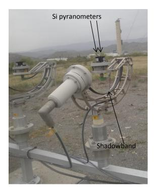
Figure 2: Twin Rotating Shadowband Irradiometer by CSP Services in resting position. The two Si pyranometers are indicated as well as the shadowband.
