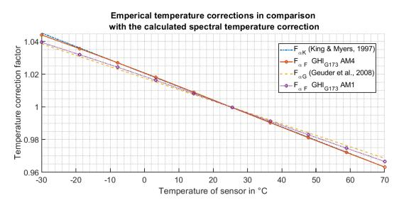
Figure 8: Spectral temperature correction factor  $F_{\alpha F}$  in comparison with currently used broadband temperature correction factors.
