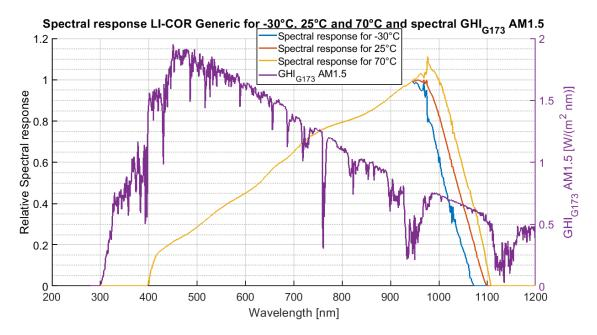
Figure 7: Calculated spectral response of the LI-200 at -30°C, 25°C and 70°C and the GHI under G173 air mass 1.5 atmospheric conditions (ASTM, 2012). The spectral response for 25°C is from (Licor, 2004) and is assumed to be 25°C as a standard laboratory temperature.
