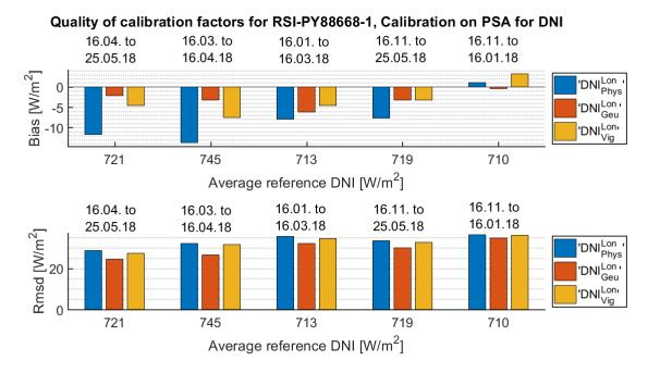
Figure 14: Absolute bias and RMSD of corrected measurements from Londrina with calibration factors from the PSA for the DNI.
