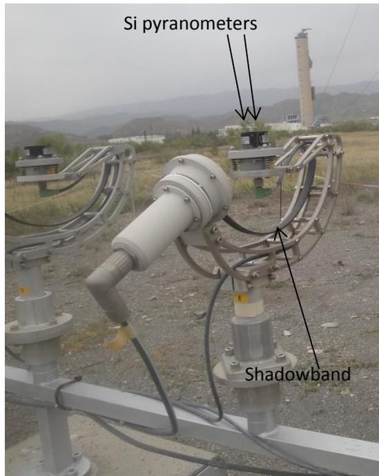
**Figure 2: Twin Rotating Shadowband Irradiometer by CSP Services in resting position. The two Si pyranometers are indicated as well as the shadowband.**
