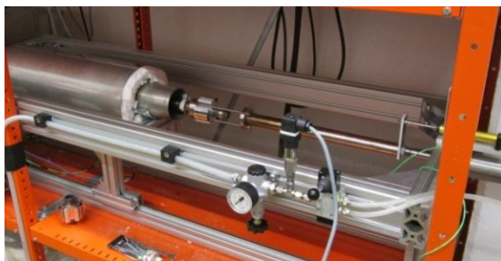
Fig. 3. Mechanical removal testing: Pulling device with tube held on the left while the pneumatic cylinder pulls the sheath the aluminum 'fin base' to the right shown, shown with the tubular oven open.
