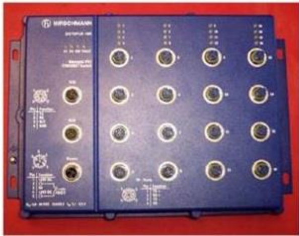
Fig. 7: The CPLSW based on a 16M Octopus Hirschmann Switch (Photo: ESA/NASA)
