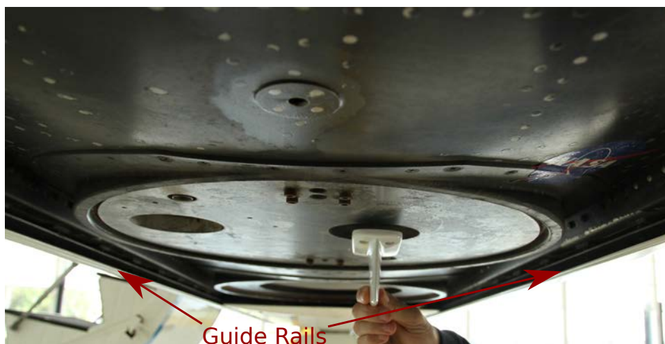
Figure B.2. Mounting of the airborne antenna on the aircraft.
