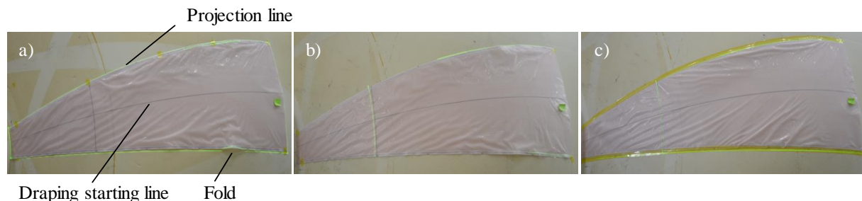
Figure 4: Deposition of Package No. 2 on 3D surface: a) punctual fixation on package contour, b) punctual fixation on outer corners, c) linear fixation on upper and lower contour
