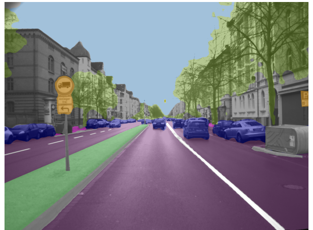
Figure 10. Example of pixel-wise annotations with 28 classes containing both static and non-static objects.
