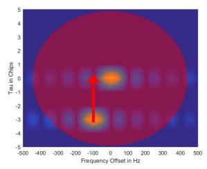
Interference forces receiver into reacquisition.
