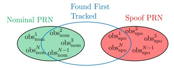
If mix is found/tracked: Allows for ARAIM based detection
