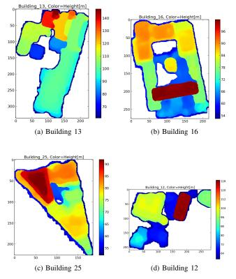
Fig. 7: Building models for processing depth level 2, color indicating height. DSM based on five WorldView-2 images.
