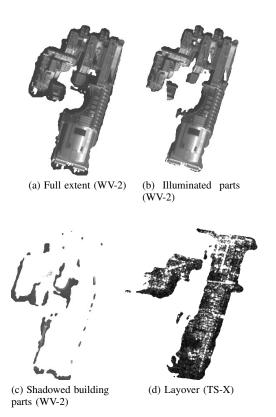
Fig. 8: Extracted image parts from WorldView-2 and TerraSAR-X images for building 13. WV-2: WorldView-2; TS-X: TerraSAR-X.
