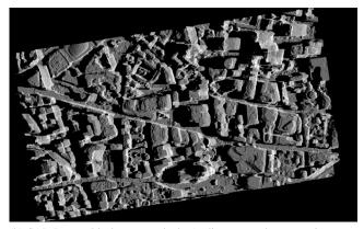
(b) SAR-Image (black: sensor shadow), distance to the sensor increases from right to left
