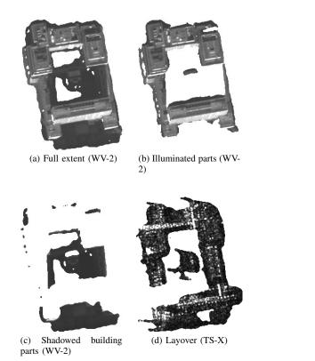
Fig. 9: Extracted image parts from WorldView-2 and TerraSAR-X images for building 16.
