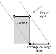
Fig. 2: Layover effect in SAR imaging due to the measurement of distance along line-of-sight. Signal contributions from roof, facade, and ground are merged for the building example.
