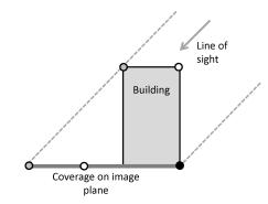
Fig. 3: Geometric projection in optical image for off-nadir angle. Facade and roof parts remain separated but are geometrically distorted.
