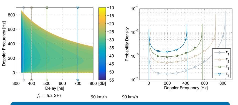
Doppler spectrum depends on delay, velocity vectors, and Tx-Rx distance
