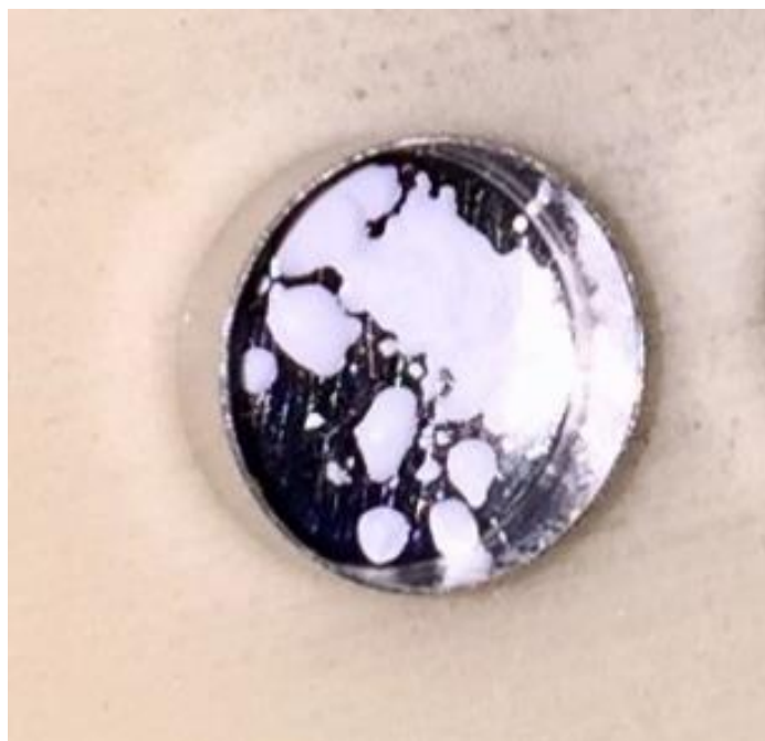
Figure S4. Molten sample after experiment 4.2 using only \text{MgCl}_2 \cdot 6\text{H}_2\text{O} .
