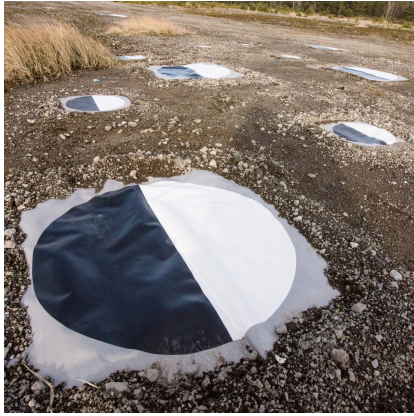
Fig. 15: Craters after preparation and ready for testing
