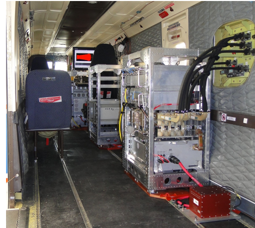
Figure 2: DBFSAR mounted in the cabin of DLR's Do228 aircraft: digital backend in the back, RF frontend in the front and X-band wave-guide connections on the very right of the image.
