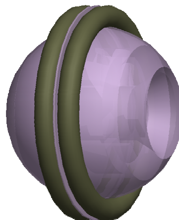
Figure 9: Double torus-like pneumatic support of the ball-shaped head providing reset forces in case of head deflection
