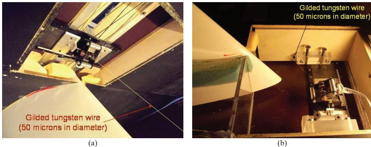
FIGURE 3. Source of freestream vortices consisted of vibrating wire in front of the airfoil leading edge driven by upper (a) and lower (b) shakers
