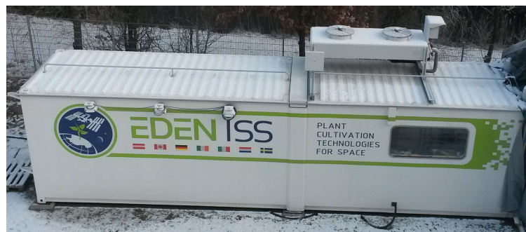
Figure 11. Mobile Test Facility with roof-mounted free cooler. Credit: DLR
