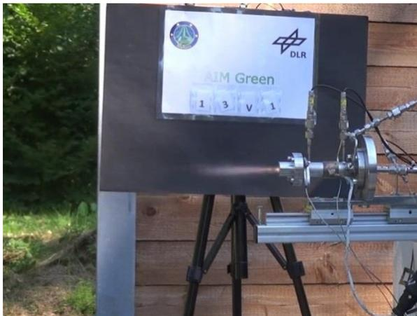
Fig. 7. Video snapshot of the ignition test with the torch igniter and additional oxygen
