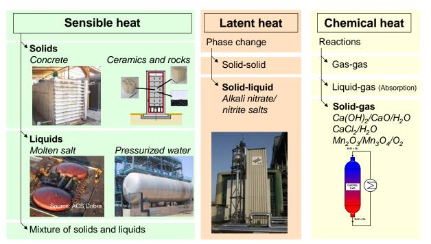
When comparing the technologies, the highest energy densities are achieved by thermochemical thermal energy storage systems, whereas sensible heat has the lowest and latent heat lies in between. However, there are reasons why the technology with the lowest energy density (sensible heat) has nonetheless achieved highest maturity and is nowadays widely applicated.
