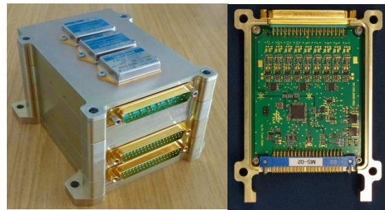
Fig. 12: High frequency data acquisition electronics box and PCB
