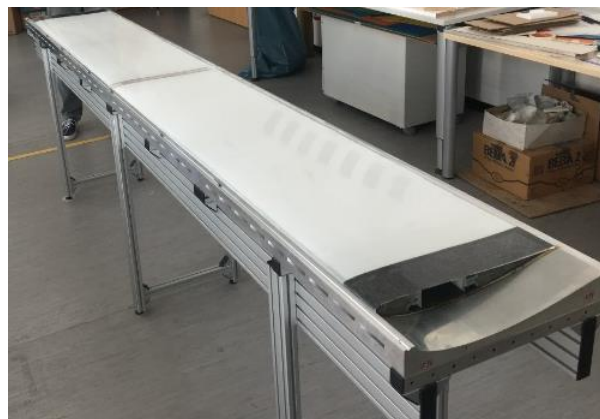
Figure 9: Mold with first finished ELAHA 10 wing-segment used for structural testing
