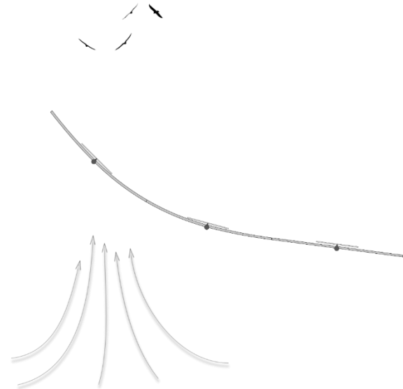
Figure 2: Thermal bending wing upwards
