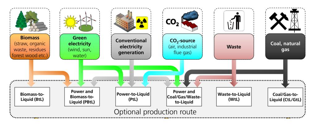
The supply of large quantities of alternative kerosene within low GHG emissions is possible by coupling the sectors renewable electricity generation and fuels *(without biomass imports).*
