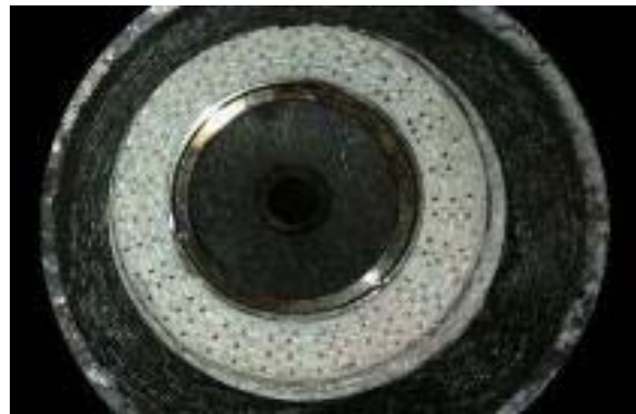
Fig. 2: Concentric cone injector face-plate with alternating ring zones for fuel and oxidiser injection.
